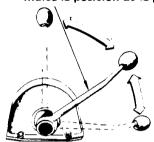
Pull out the knob for engine warm-up and place the control lever in the "half speed" position.
